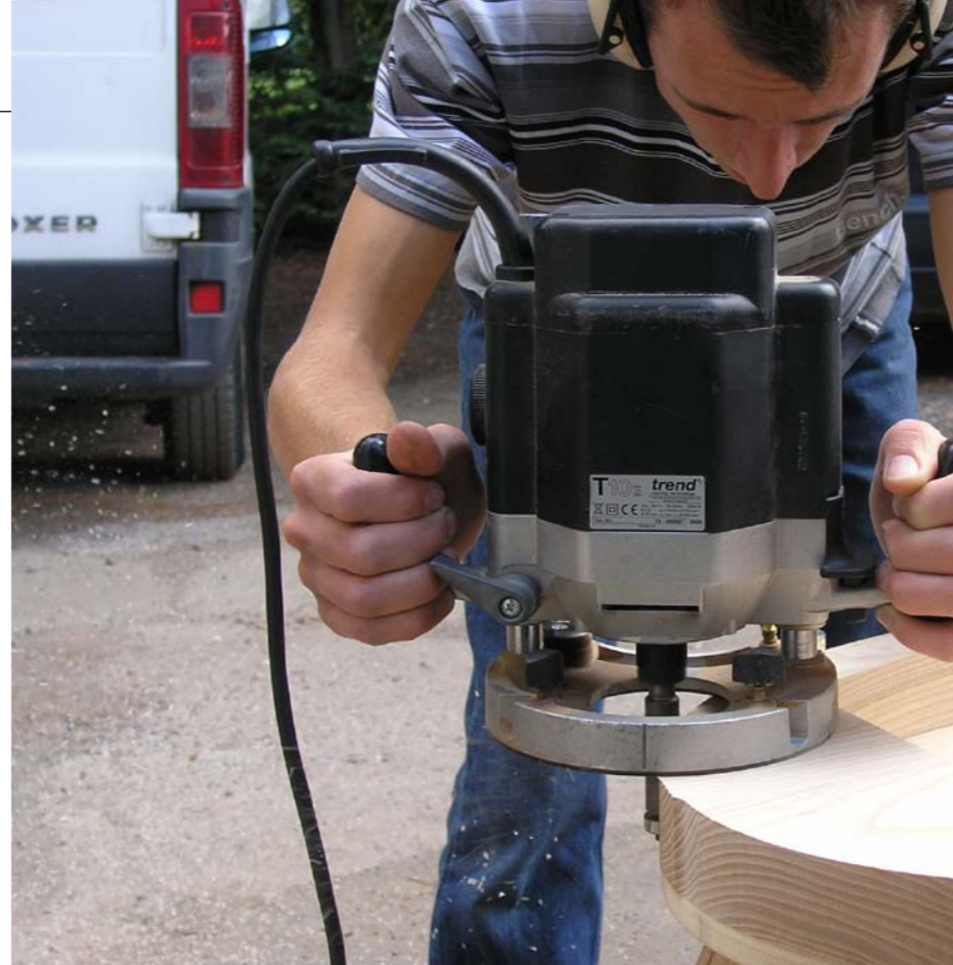
Pic.4 Routing the hoops roughly to shape with a template (left) and using a power planer (above) to smooth the base. In the end a disc sander proved to be best option. Charlie used the narrowest part of each hoop as a guide for depth and never went below that point
