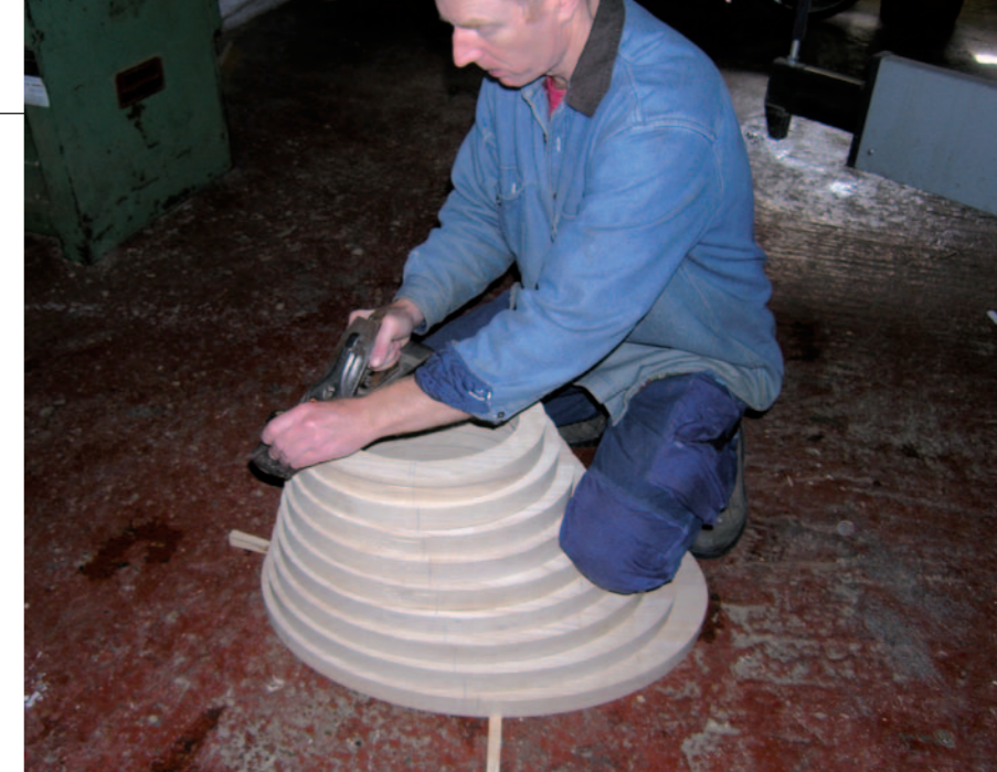
Pic.2 Drilling the steel plate that fixes the base to the top (above left), and planing the part-assembled base (above) for the next layers to be glue in place (below)
