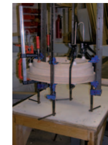
Pic.2 Drilling the steel plate that fixes the base to the top (above left), and planing the part-assembled base (above) for the next layers to be glue in place (below)
