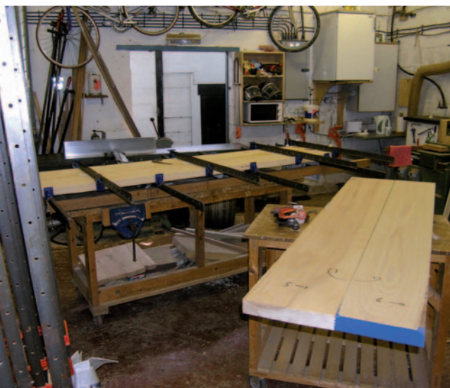
Pic.3 With careful nesting the hoops were cut from three large ash boards (above). Once they had been CNC'ed to shape they were stacked up in threes. Charlie used abrasive stuck down on a saw table to level the stack
