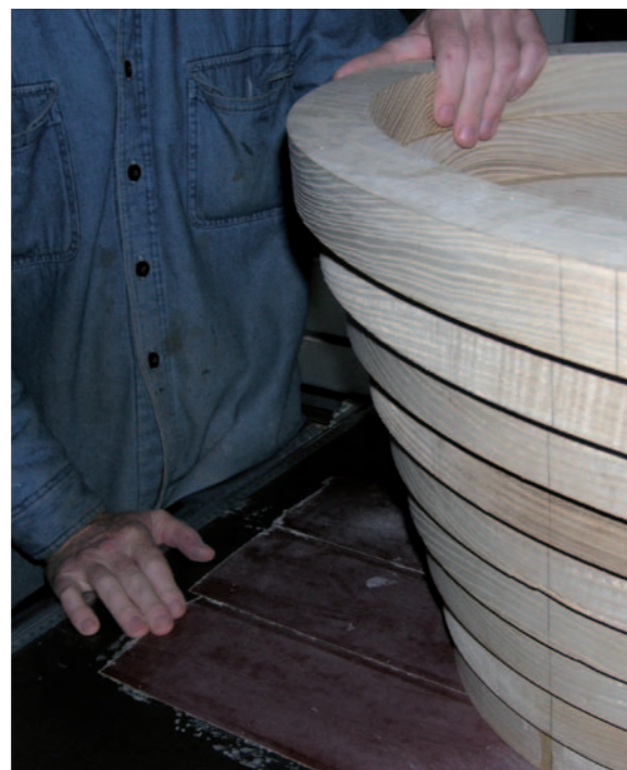
Pic.3 With careful nesting the hoops were cut from three large ash boards (above). Once they had been CNC'ed to shape they were stacked up in threes. Charlie used abrasive stuck down on a saw table to level the stack
