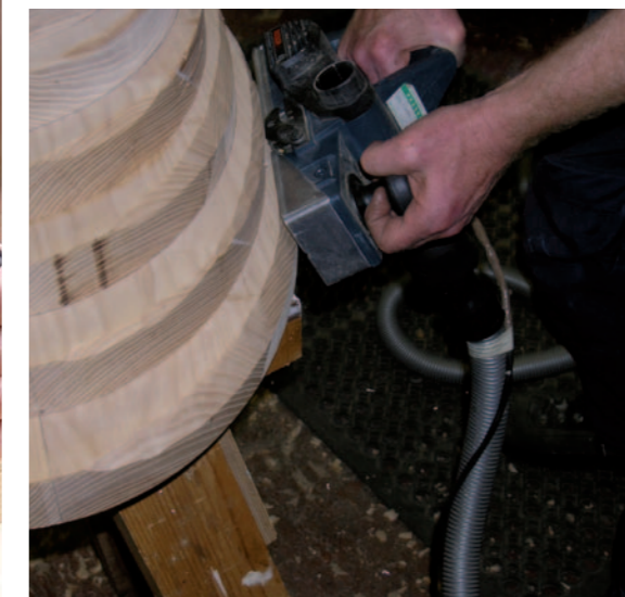
Pic.4 Routing the hoops roughly to shape with a template (left) and using a power planer (above) to smooth the base. In the end a disc sander proved to be best option. Charlie used the narrowest part of each hoop as a guide for depth and never went below that point
