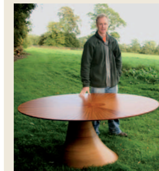
Pic.5 There are similarities in texture and grain between ash and zebrano, so with some stain Charlie was able to make a zebrano-style base to meet a budget that called for American ash.
